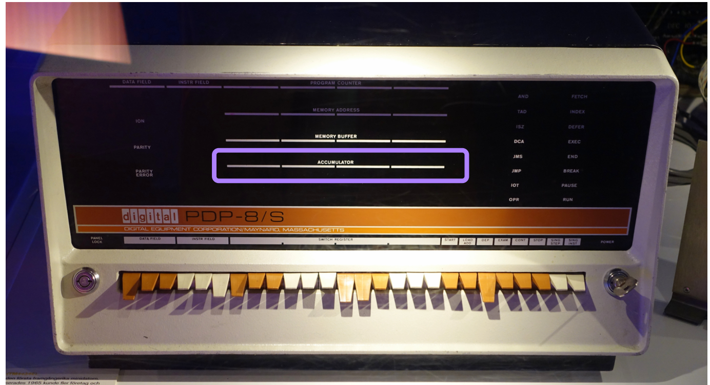
Digital Equipment Corporation (DEC) PDP-8, 12-bit accumulator architecture, 1965.
